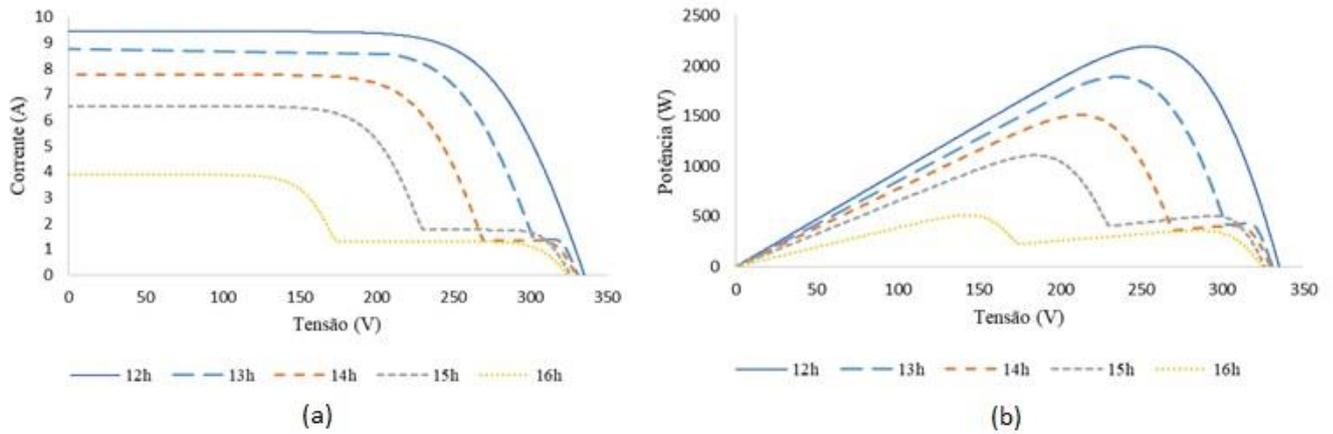
Figura 16 – (a) curva  $I-V$ ; (b) curva  $P-V$  modeladas no Crearray.
