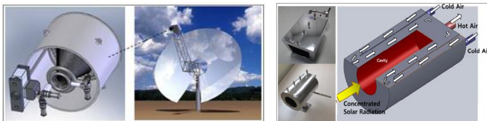
Figure 2- (a) SolarCAT system developed by SolarCAT Inc. company and (b) solar receiver developed by Kim et al. (2014).
