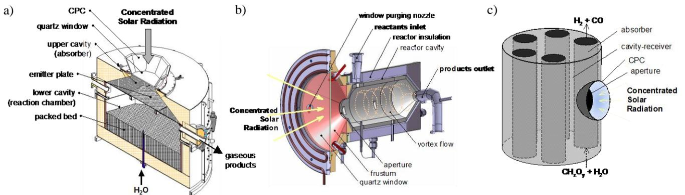
Fig. 1. Solar reactor configurations for the steam-based thermochemical gasification of carbonaceous feedstocks: a) indirectly-irradiated packed-bed reactor; b) directly-irradiated vortex-flow reactor; and c) indirectly-irradiated entrained-flow reactor.
