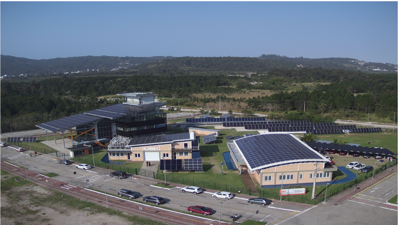
Figure 2 – The Fotovoltaica/UFSC solar energy research laboratory, with the green H 2 laboratory building, which collects rainwater, produces solar electricity and houses the electrolysis system shown in the left-hand corner.
