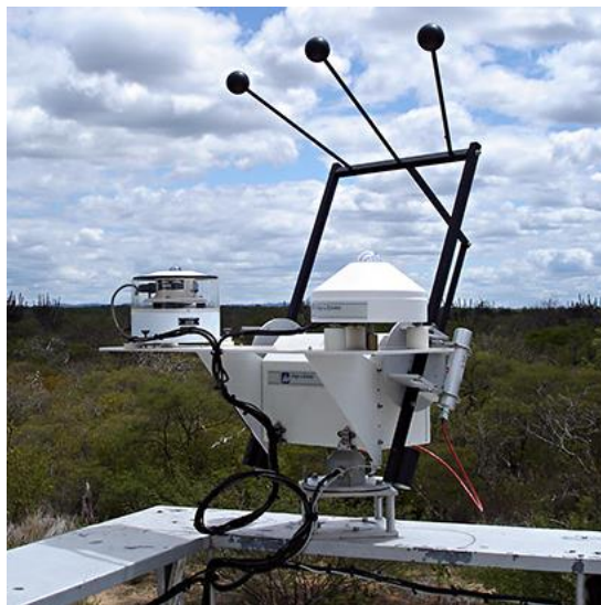
Figure 1 - Petrolina SONDA Solarimetric Station solar tracker, with two pyranometers, one pyr heliometer, and shadow ball equipment.
