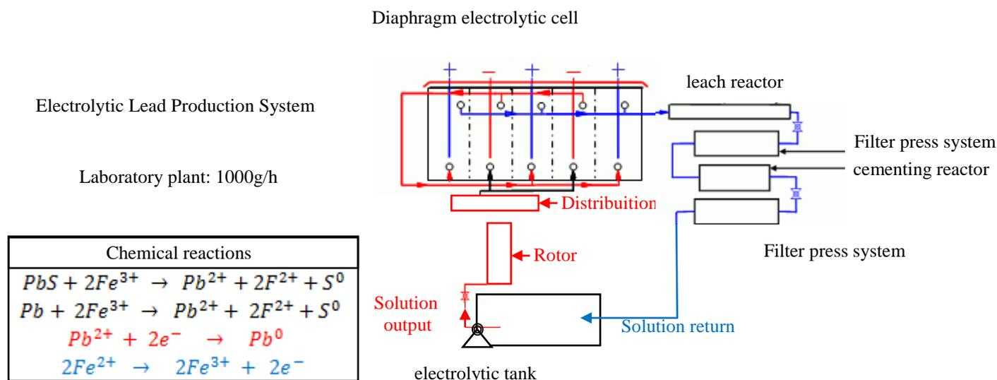
Figure 3 Schematic of the electrohydrometallurgical process of lead production (Electrolytic cell in Polyvinyl chloride machined - Electrolyte tank - Polyvinyl chloride pipes)
