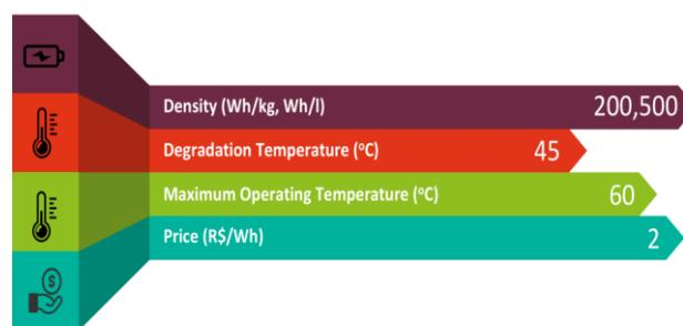
Figure 2 - Characteristics of lithium-ion battery
